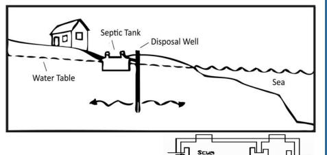
the bottom, forming a sludge layer; grease, fats and hair float to the top, forming a scum layer; between these two layers is the liquid effluent which flows to the disposal well.
